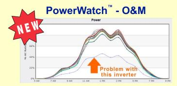
PowerWatch compares all inverter outputs to identify a faulty inverter. 30 day energy ratio log tracks intermittent operation.
